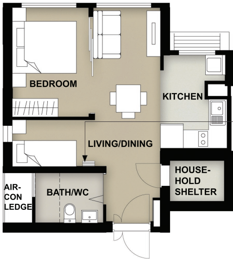
2-ROOM FLEXI (TYPE 2) FLOOR PLAN (With Suggested Furniture Layout) Approx. Floor Area 48sqm Inclusive of Internal Floor Area of 46sqm and Air-con Ledge
