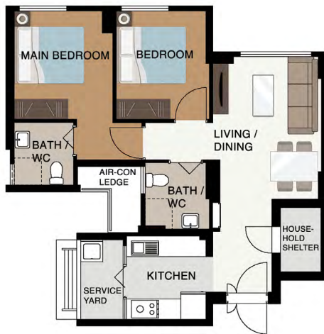
3-ROOM FLOOR PLAN (With Suggested Furniture Layout) APPROX. FLOOR AREA 69 sqm (Inclusive of Internal Floor Area of 66 sqm and Air-Con Ledge)
